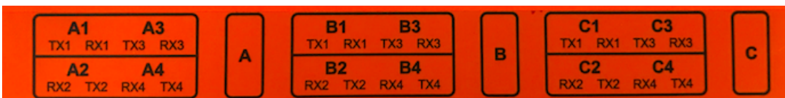
Figure 19 Port Label for Breakout Panels PNL-M341, PNL-M341T, PNL-M343, and PNL-M343T
